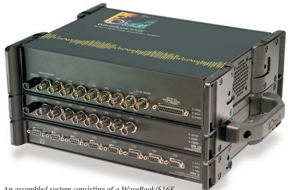
An assembled system consisting of a WaveBook/516E plus one WBK18 accelerometer module plus one WBK16 strain gage module
