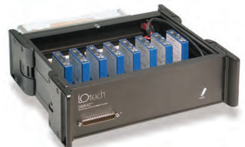
DBK42 with installed 5B modules
