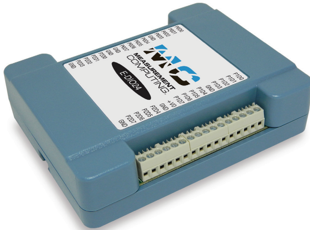
The E-DIO24 provides 24 lines of digital I/O with \pm 24 mA drive capability
