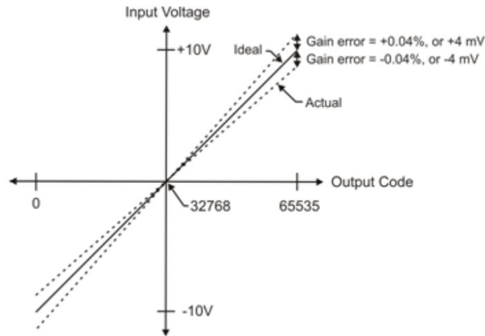
Figure 9. ADC Transfer function with gain error
