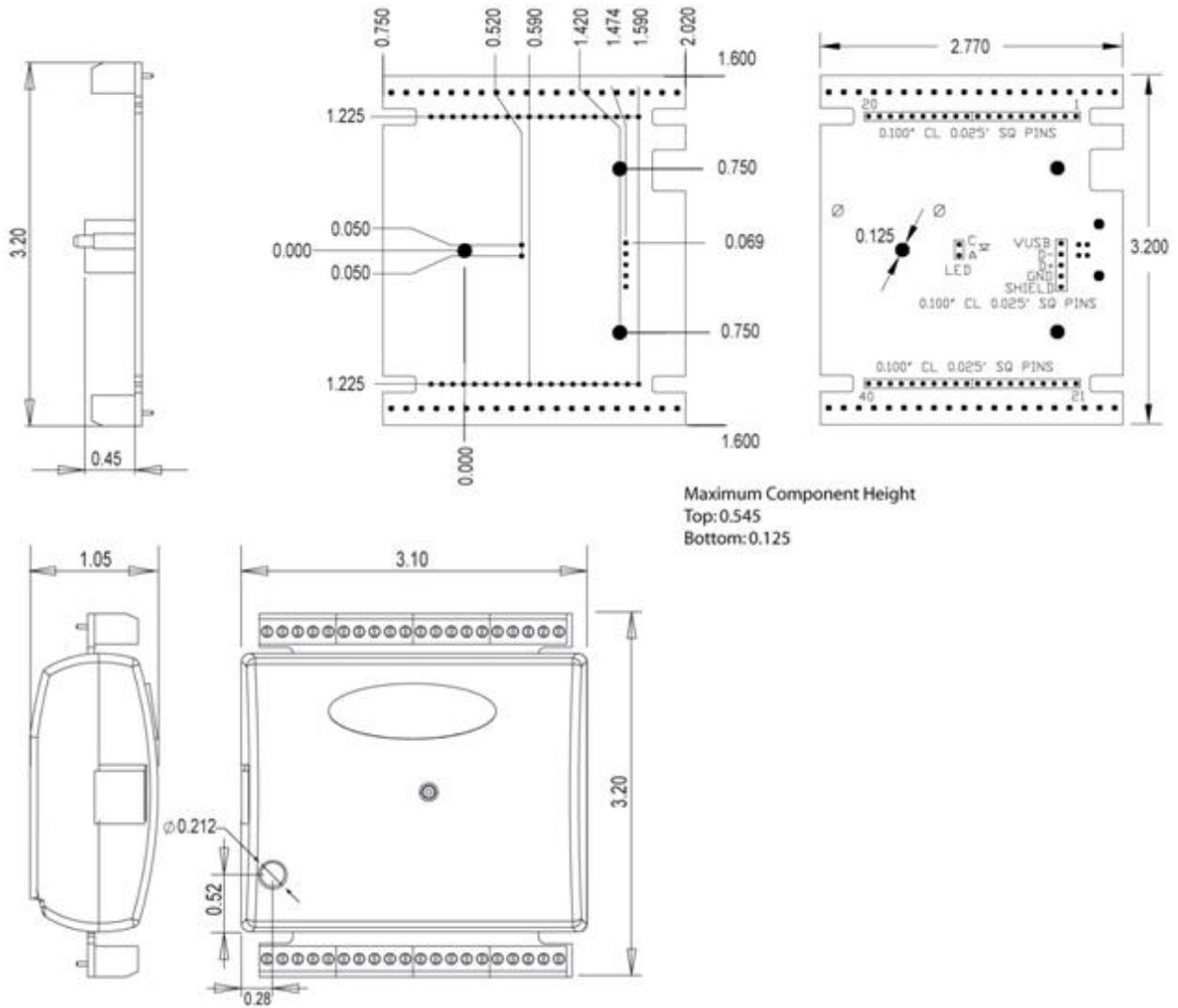
Figure 11. USB-1608FS-Plus circuit board (top) and enclosure dimensions
