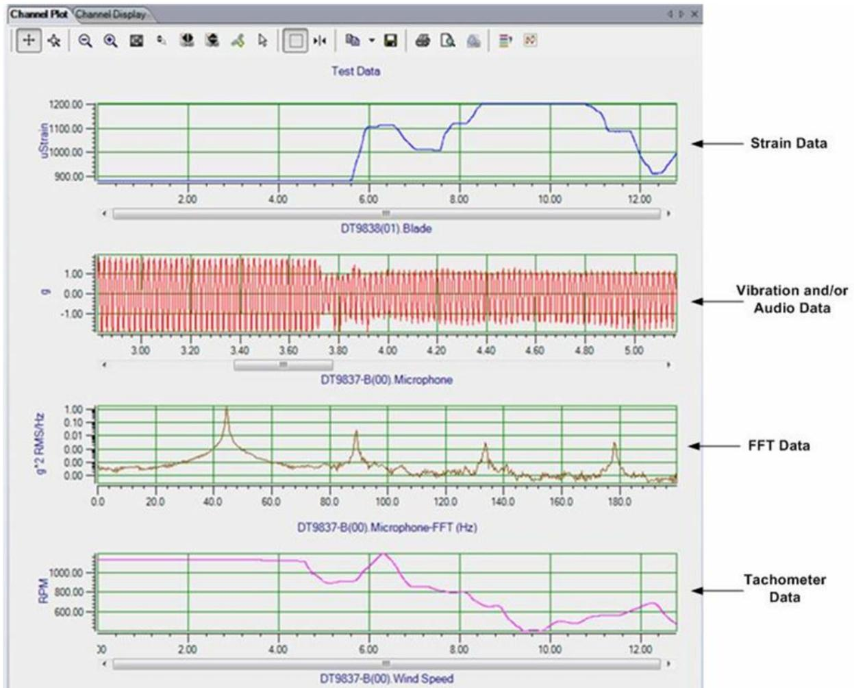
Figure 2. Easy configuration of multiple sensor types allows one to acquire and view vibration, strain, and tachometer data together.
