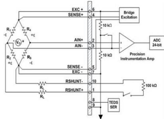
For strain measurements, use a device that supports the required bridge configurations with bridge completion, proper excitation, and Transducer Electronic Data Sheet (TEDS) smart sensor compatibility like the DT9838 from Data Translation.
