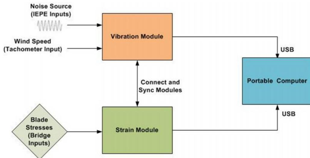
Figure 1. Synchronizing multiple sensors and devices allows users to capture vibration, strain, and tachometer signals all correlated precisely in time – critical for diagnosing operating issues.
