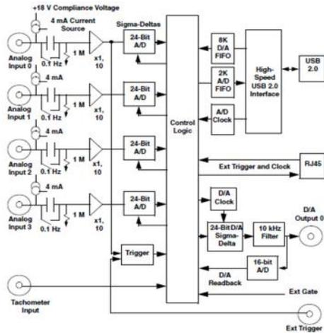
For vibration measurement, use a device that accommodates direct connection of IEPE inputs and provides the proper current and coupling requirements like the DT9837 Series from Data Translation.
