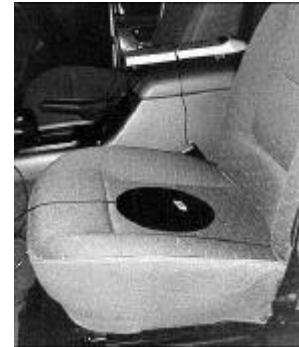
Fig. 1: Triaxial accelerometer sensor used for WBV measurement
